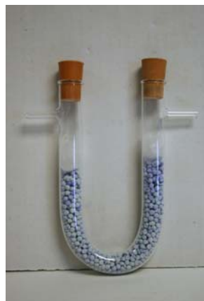
Fig. 5. 15g LoFloSorb desiccated by oxygen
