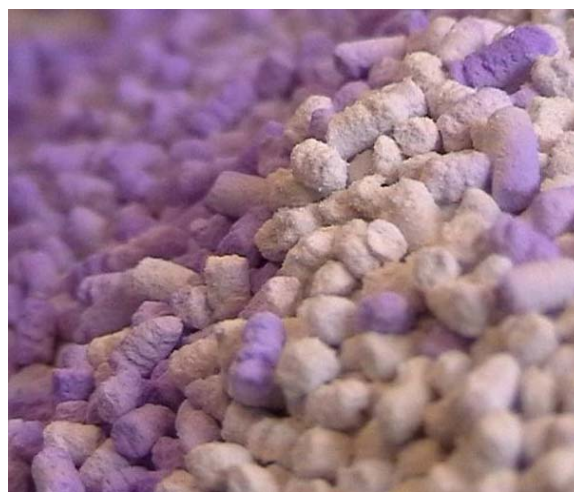
Fig. 1. Fresh AMSORB PLUS (white coloured) and desiccated AMSORB PLUS (violet coloured)
