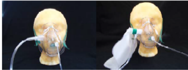
Figure 2 showing a picture of the set ups used during testing. The medium concentration adapter configuration is showed on the left, the high concentration adapter configuration is showed on the right.
