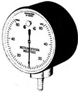
#GZ-NS60-PBS Gauge reads \pm 60\text{cm H}_2\text{O} in 2cm dial markings with 1/8" small bore tubing connection on bottom..
